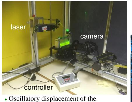
• Oscillatory displacement of the suspension in simple shear flow.
