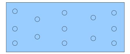
• Subdivide the bulk sample to prepare several analytical samples. It will be statistically poor. Better to sample the flowing stream when the wagon or box is being filled.
