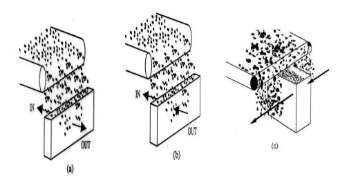
**Sampling from falling conveyors:** (a) bad sampling technique, (b) good sampling technique, (c) sampling procedure to be adopted for high mass flow rat (Courtesy of Reg Davies, 2009).
