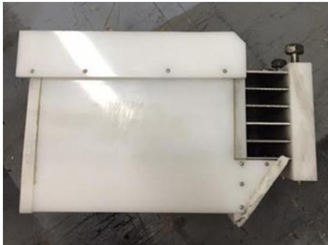
Designed & fabricated froth sampler to obtain composition as a function of depth
