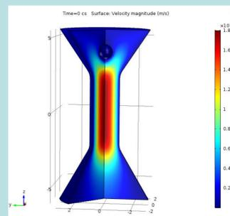
Velocity profile around charged particle in a converging-diverging channel
